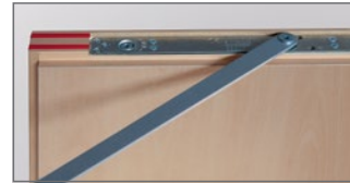
DC 840 covered door closer with slide rail (non-rebated door)
